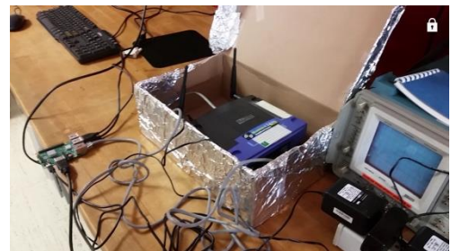
Figure 4.1.1: Com Setup inside Faraday Cage
