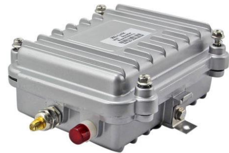
Figure 3.1.7: 2.4 GHz Power Amplifier B
